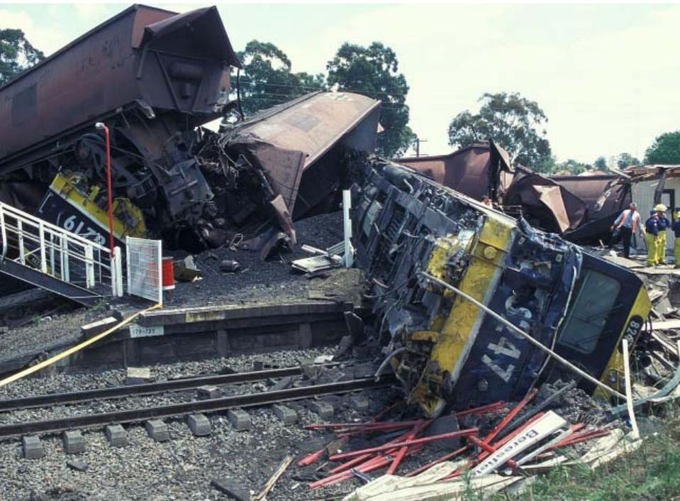
The Bureau of Air Safety Investigation (BASI) inquiry into the collision between a moving and a stationary coal train at Beresfield (NSW) in October 1997 found that fatigue from rotating shift work and broken sleep patterns were major factors contributing to the collision. The limitations of conventional vigilance control systems were also highlighted during the investigation. Richard Whitford
